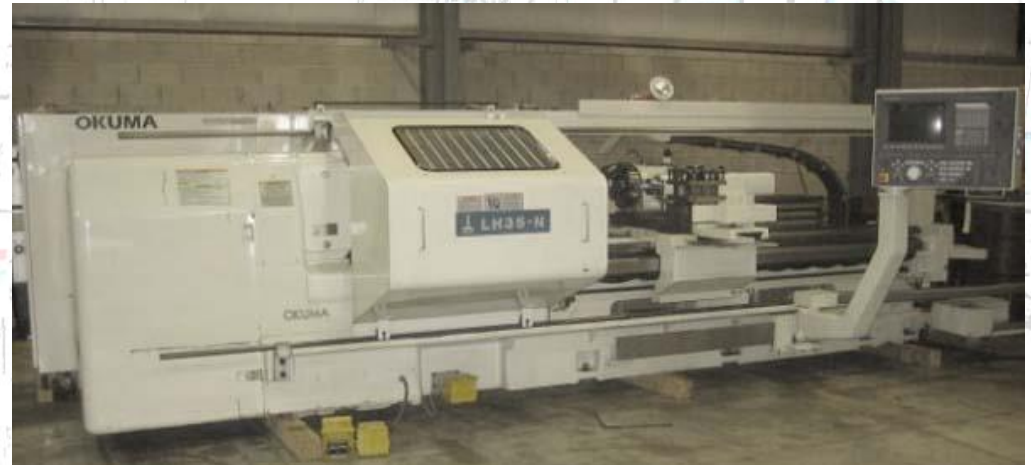
CNC LATHE OKUMA LH35N = 1 MACHINE Machining Cap Ø300 X 3000
