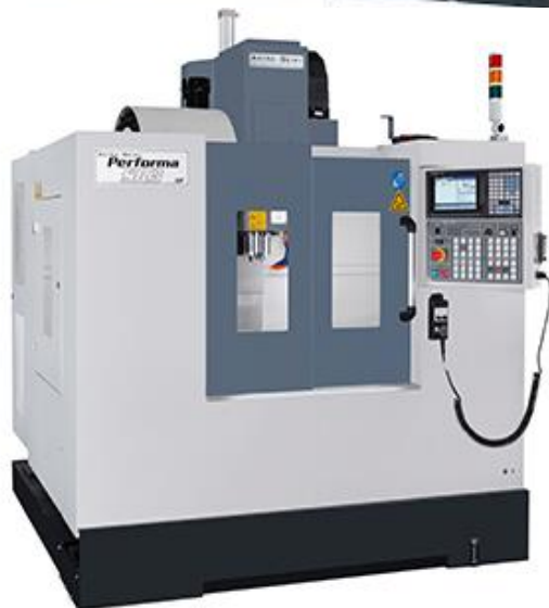
CNC → AKIRA PERFORMA = 1 MACHINE 760 X 400 X 440
